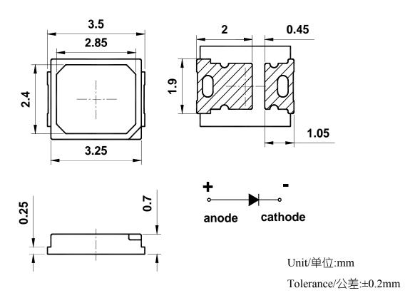
Electrodes/焊盘: Ag Plating/银
