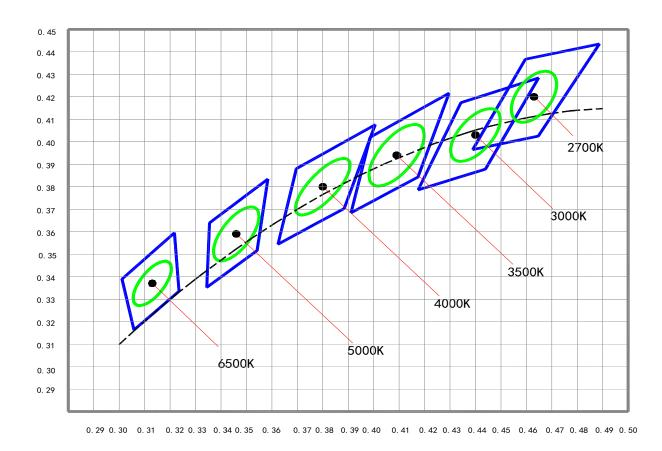
Shooting figure based on IEC60081 color tolerance standard coordinates/按IEC60081色容差
