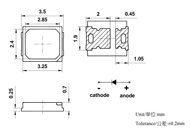
Electrodes/焊盘: Ag Plating/银
